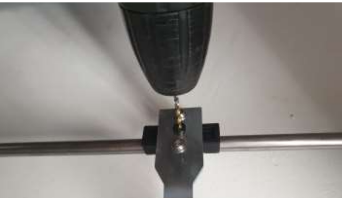
Best velocity for drilling is 2600 rpm Remember to lubricate drill often
