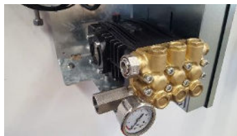
The pump is ready for demounting
