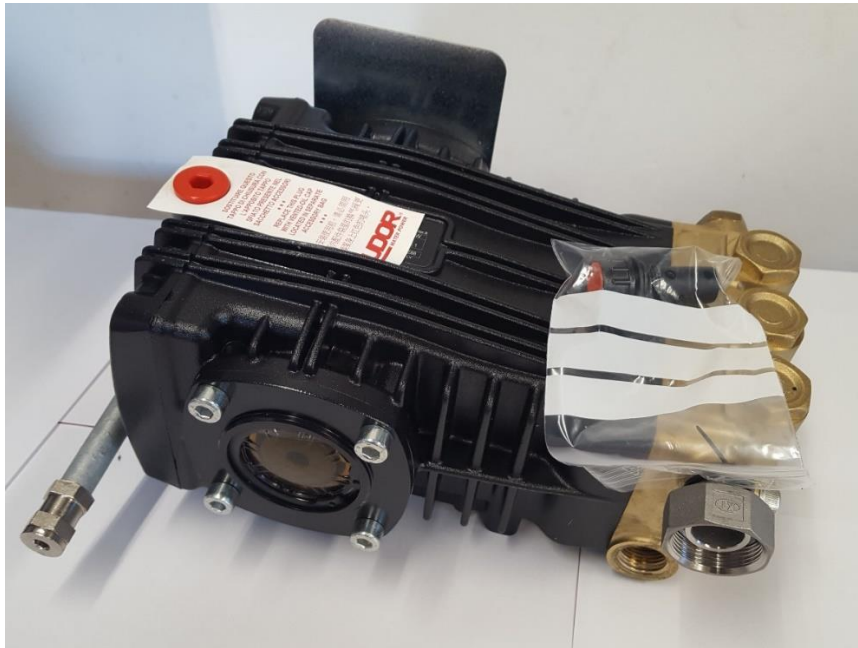
View of the replacement pump
